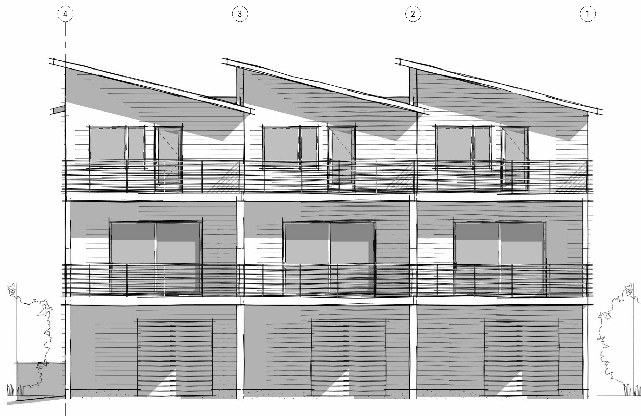
③ SOUTH ELEVATION 3/16" = 1'-0"
